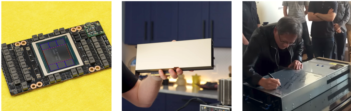
Figure 2. Left, an Nvidia H100 printed circuit board, without casing, with the GH100 GPU (outlined in red) and six surrounding high-bandwidth memory chips (outlined in blue) in the center (source: CNET ). Middle, an Nvidia A100 accelerator, with casing (source: Linus Tech Tips ). Right, Jensen Huang, president and CEO of Nvidia, signing the first delivered Nvidia DGX server (source: Nvidia ).
